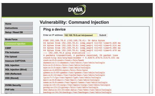
FIGURE 6-14 Example of a Command Injection Vulnerability
