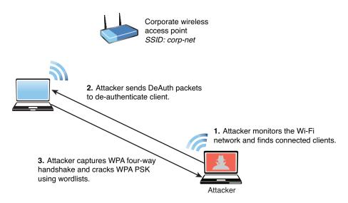
FIGURE 5-20 Capturing the WPA Four-Way Handshake and Cracking the PSK
