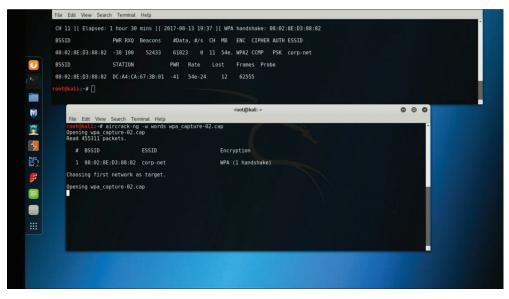
FIGURE 5-23 Collecting the WPA Handshake Using Airodump-ng
