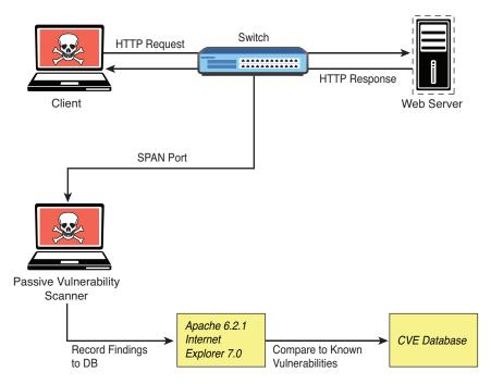
FIGURE 3-16 Passive Vulnerability Scanner Diagram
