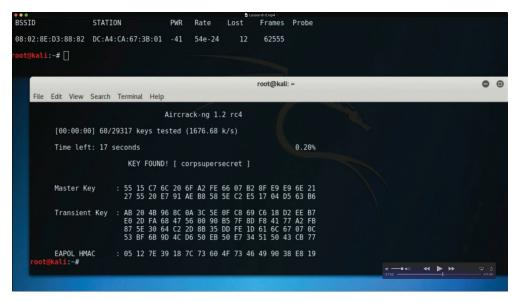
FIGURE 5-24 Cracking the WPA PSK Using Aircrack-ng
