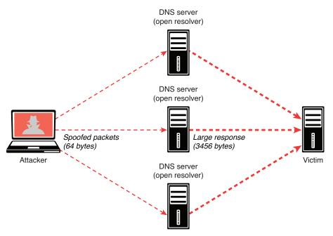
FIGURE 5-10 DNS Amplification Attack
