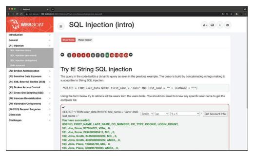
FIGURE 6-9 Example of a Basic SQL Injection Attack Using String-Based User Input
