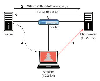
FIGURE 5-2 DNS Cache Poisoning Example
