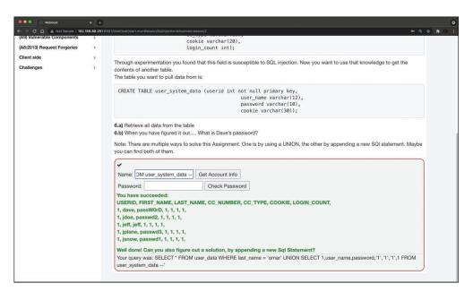
FIGURE 6-11 Example of a UNION Operand in an SQL Injection Attack
